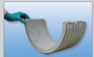
Apply filler thickly to both half casings and press in spacer (distance to half casings 5 mm)
