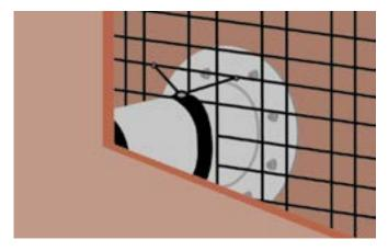
Fasten pipe clip to steel casing by means of welded joints (pipe clip on site).
