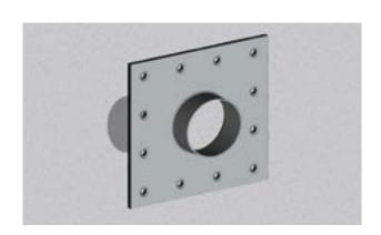
2. Remove sleeve from the wall and bore holes.
