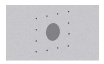
3. Apply included sealing compound on the backside of sleeve (in thick stripes Ø 6 mm − 10 mm), one stripe between the outside edge of flange and screwhole. An other one between welded sleeve and screwhole. Put last stripe around the screwhole.
