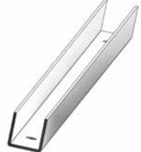
Guiding rail (concrete casing pipe)
