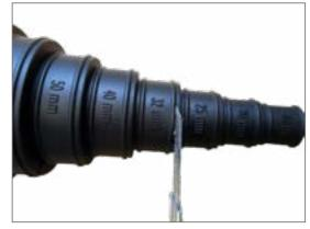
Prepare casing end seal suitable for medium pipe size. Cut off with a sharp knife between the marking and the end of the step.
