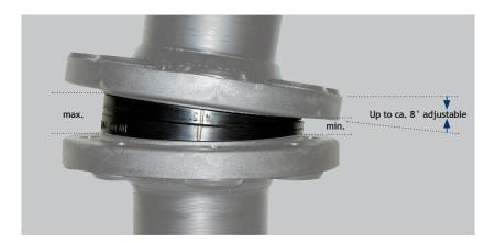
The standard material of the PSI adjustable flange gasket WD is EPDM. However, depending on the application, it can also be made of other elastomers such as FPM (Viton) and silicone. EPDM service temperature ranges from -25 °C to +120 °C
