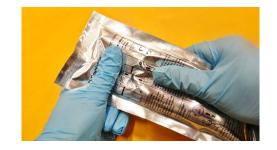
**<u>3. Initial Mixing</u>** With a gloved hand, mix the contents together by kneading the Covalence Epoxy Twin Pack. Make sure to work out the material from the corners.
