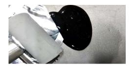
5. Opening of the Twin Pack Wear disposable gloves and, using a knife or scissors cut the corner of the pack.Gradually squeeze the content of the package out onto the pre-heated steel surface. Be careful as the content may be hot!
